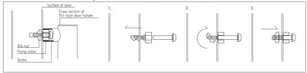
O Drill 1/2inch hole through the door surface. Set the rib nut in the hole. Insert the screw into the fixing collar. Then, gradually tighten the rib nut and the fixing collar.
