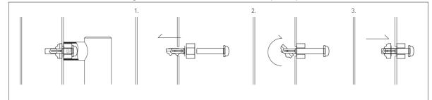
① Drill 1/2inch hole through the door surface. Set the rib nut in the hole. Insert the screw into the fixing collar. Then, gradually tighten the rib nut and the fixing collar.
