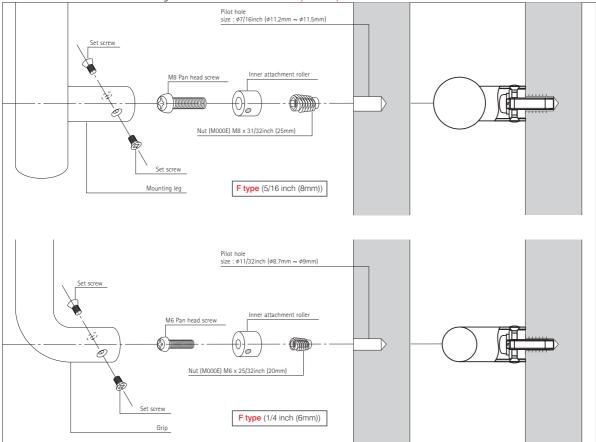
Thread insert for concealed fixing hardware on wood door Optional parts
