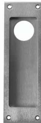
C-90C - Flush Pull with Cylinder hole supplied with Cylinder: 1" [25.4mm] Diameter hole x 1" [25.4mm] depth. 5-PIN Schlage "C" Key way
